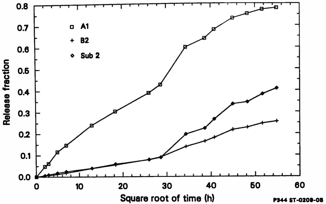
Figure 9. Cumulative <sup>137</sup>Cs release fractions relative to leaching time.
