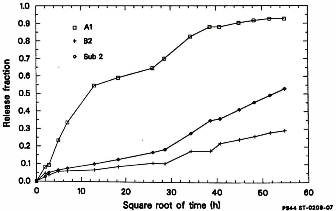
Figure 10. Cumulative <sup>90</sup>Sr release fractions relative to leaching time.
