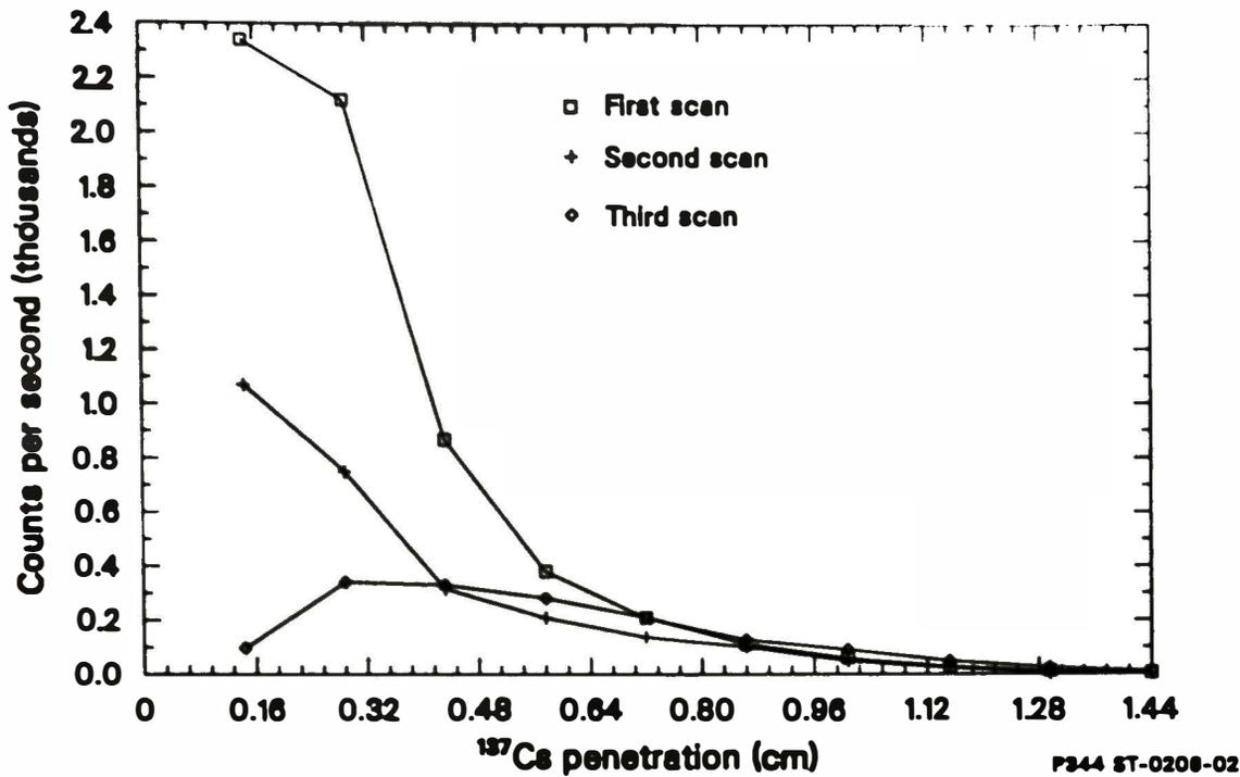
Figure 6.  $^{137}\text{Cs}$  penetration in the 3000-psi concrete (A1).
